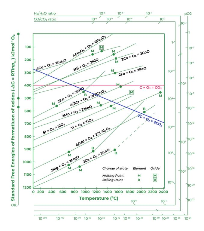
It is a free energy data that graphically plot  $\Delta G^{\circ}$  vs T for compound (oxide).
