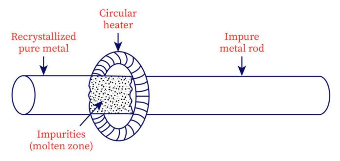
Zone refining, also known as zone melting, is a high-purity metal purification technique based on the principle of fractional crystallization. It is primarily used to refine semiconductors (such as silicon and germanium) and metals (like gallium, indium, and zirconium) where ultra-high purity is required.
